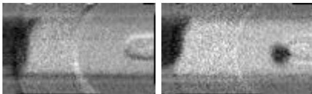
Figure 1. STXM images before and after nucleation of a skyrmion at a 500 nm wide point contact to a Pt/CoB/Ir multilayer.
