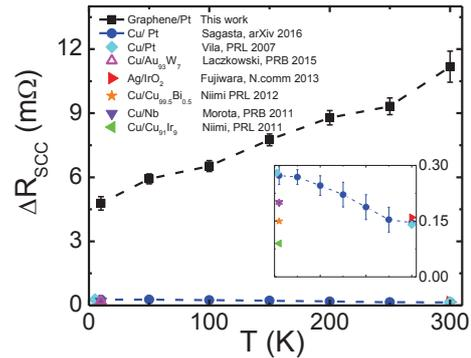
Fig. 2: Experimentally measured  $\Delta R_{SCC}$  as a function of temperature for different spin Hall metals employing different spin channels. Inset: Zoom of the previous plot showing the data of the devices with metallic spin channels.
