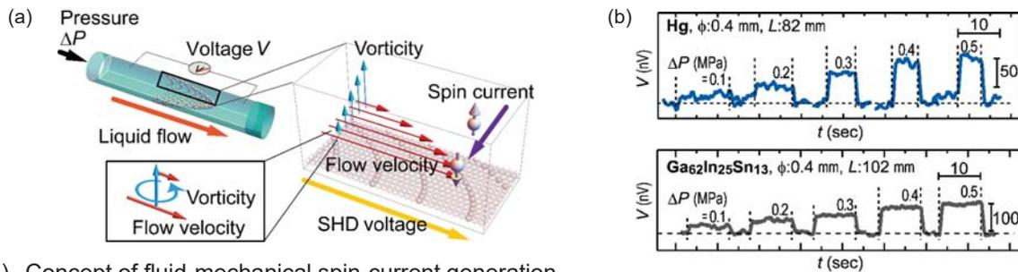
(a) Concept of fluid-mechanical spin-current generation.
