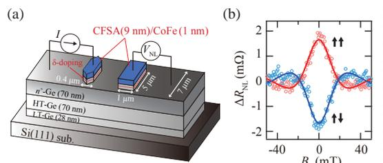
Fig. 1 (a) Schematic of a Co<sub>2</sub>FeSi<sub>0.5</sub>Al<sub>0.5</sub>/CoFe/n<sup>+</sup>-Ge LSV. (b) Nonlocal Hanle effect curves at 8 K.
