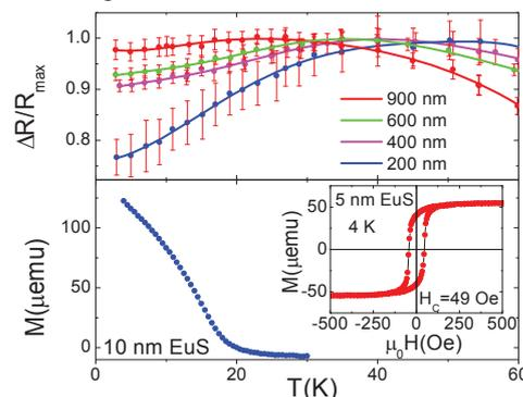
(b) Temperature dependence of normalized NLSV signal for different injector-to-detector distances (c) Temperature and field dependence of magnetization for 10 nm and 5 nm thick EuS film, respectively.
