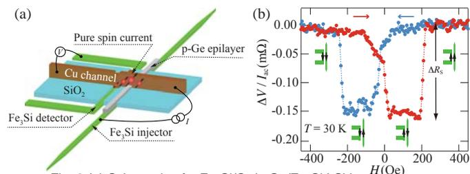
Fig. 2 (a) Schematic of a Fe<sub>3</sub>Si/Cu/p-Ge/Fe<sub>3</sub>Si LSV. (b) A nonlocal magnetoresistance curve at 30 K.
