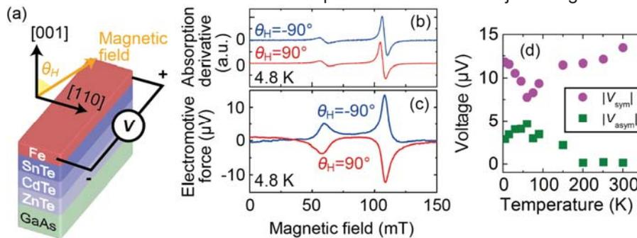
FIG. 1 (a) Schematic illustration of the device structure and the measurement alignment used in this study. (b)(c) Absorption derivative (b) and the EMF (c) as a function of a magnetic field at 4.8 K. (d) Temperature dependence of  $|V_{\text{sym}}|$  and  $|V_{\text{asym}}|$  with the magnetic field direction  $\theta_H = 90^\circ$ .
