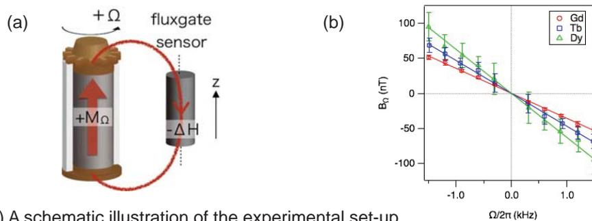
(a) A schematic illustration of the experimental set-up.
